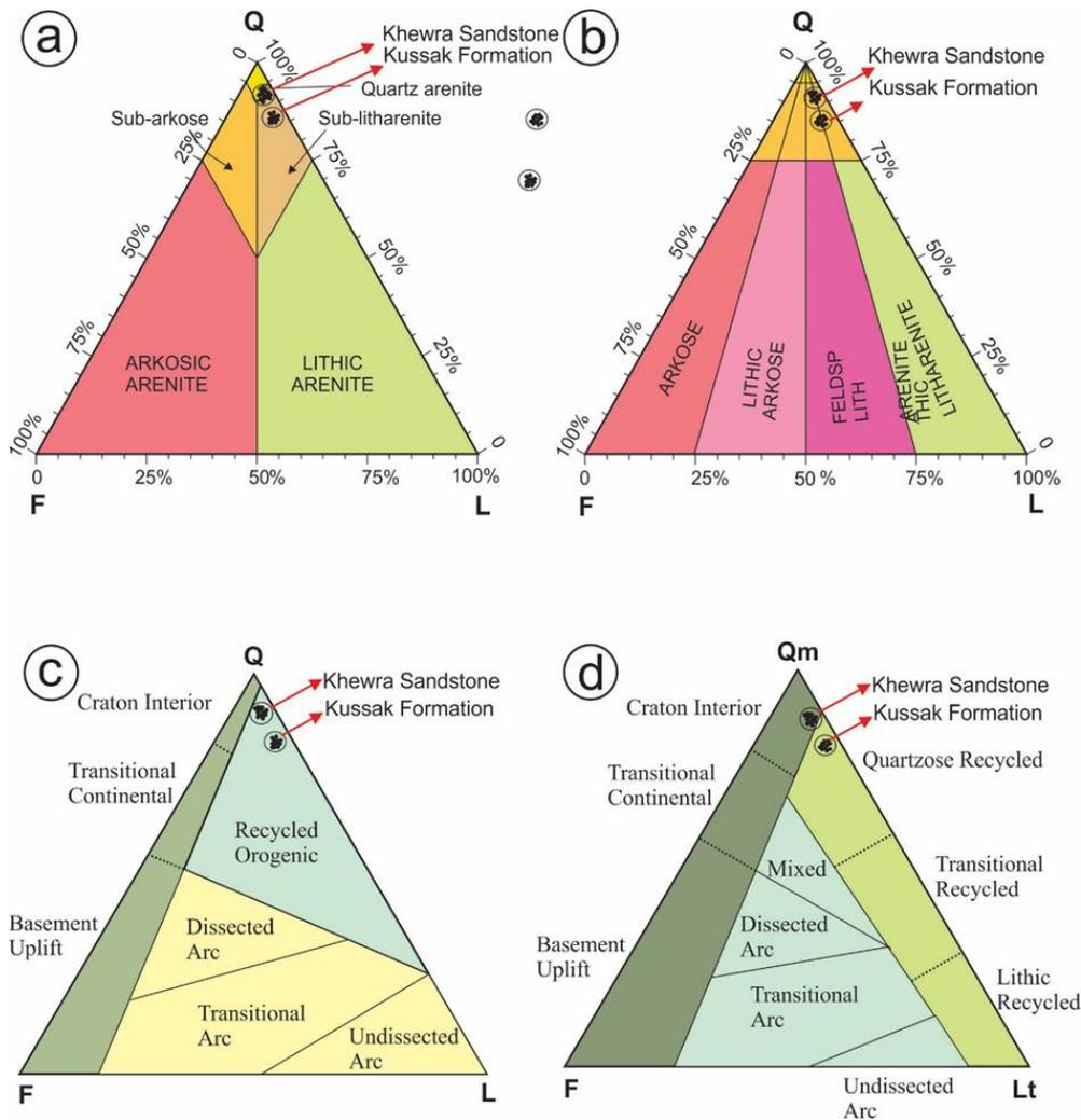
Figure 11 Interpretation of the sandstone composition from the petrography of the Khewra and Kussak Formation, showing the composition, classification as well as the suggested provenance areas for the studied thin sections. (a) QFL diagram based on the scheme of Pettijohn (1975), (b) QFL diagram based on the scheme of Folk (1980), (c and d) are modified from Dickinson and Suczek, (1979); Dickinson et al., (1983).
