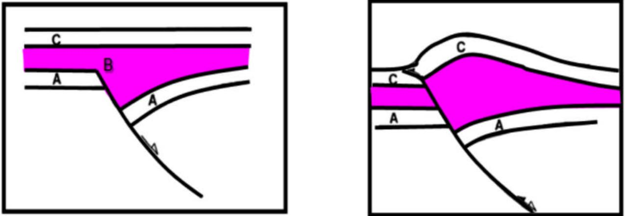
Figure 6 - Model showing geometry of positive inversion structures.
