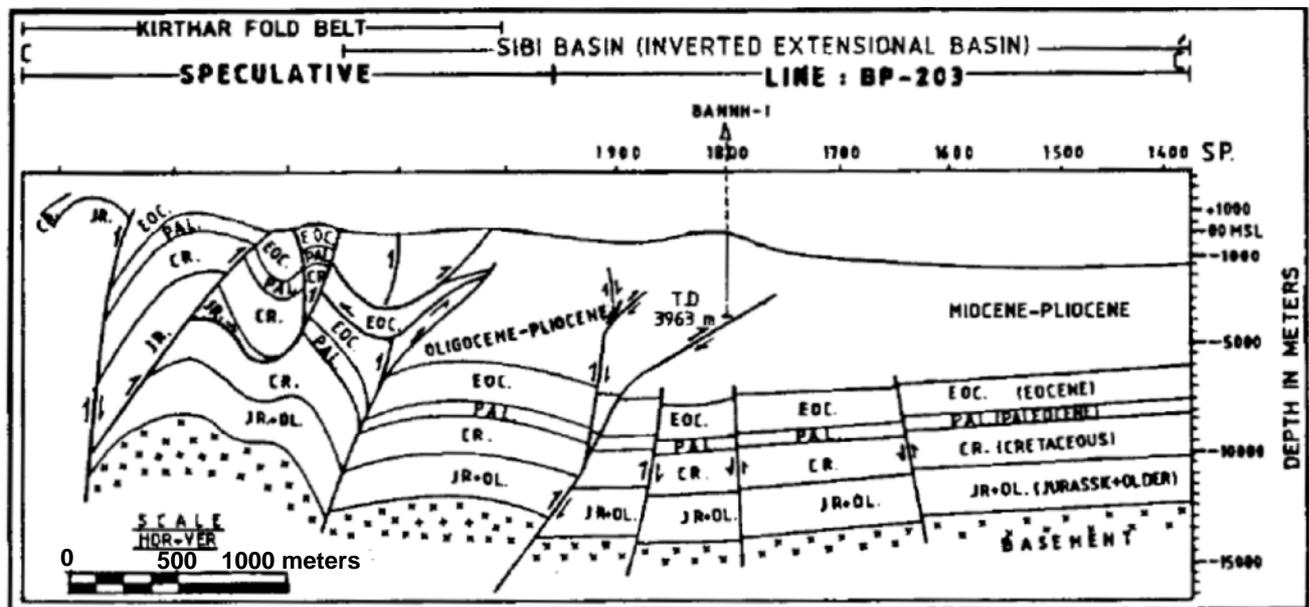
Figure 10 - Structural cross-section across Bannh well in Sibi basin showing inversion of pre-existing normal faults of Mesozoic rift to high angle reverse faults (after Ahmed et al., 1991).
