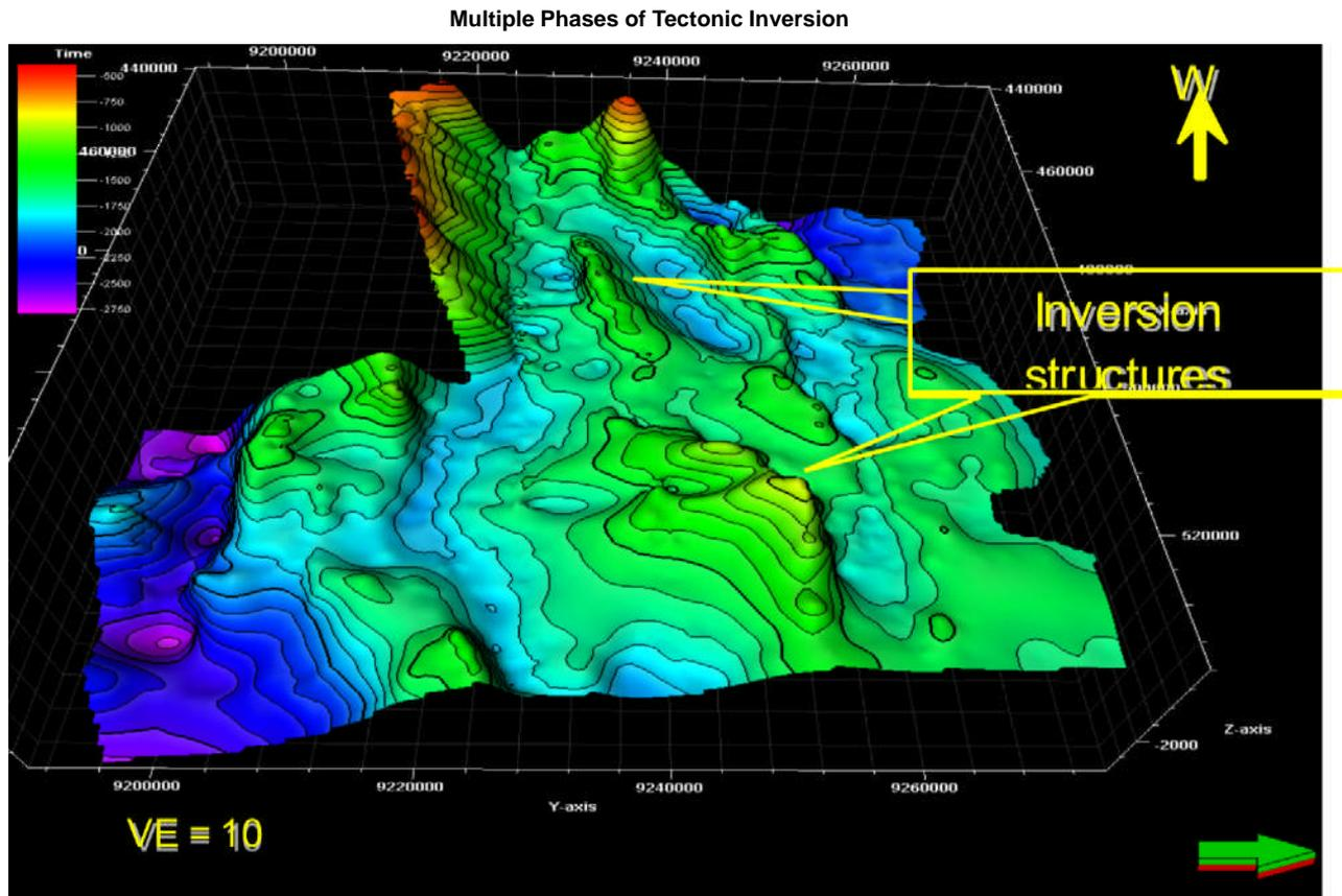
**Figure 8 -Time contour surface at top M2 level showing the geometry of positive inversion structures.**
