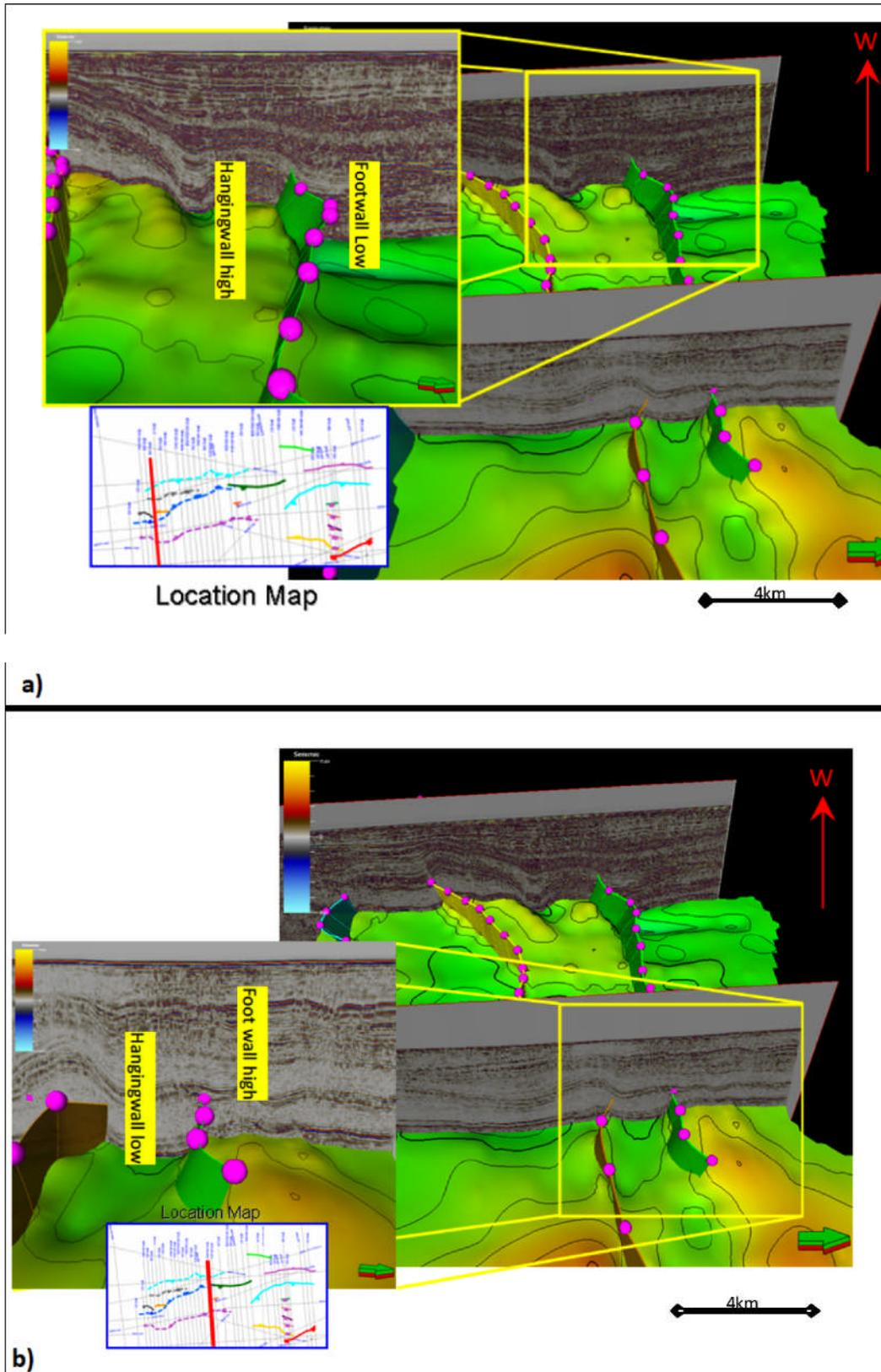
Figure 9 -3D surface, showing the reversal of throw along strike of the fault at top Cretaceous level in EW direction across the northern basin.
