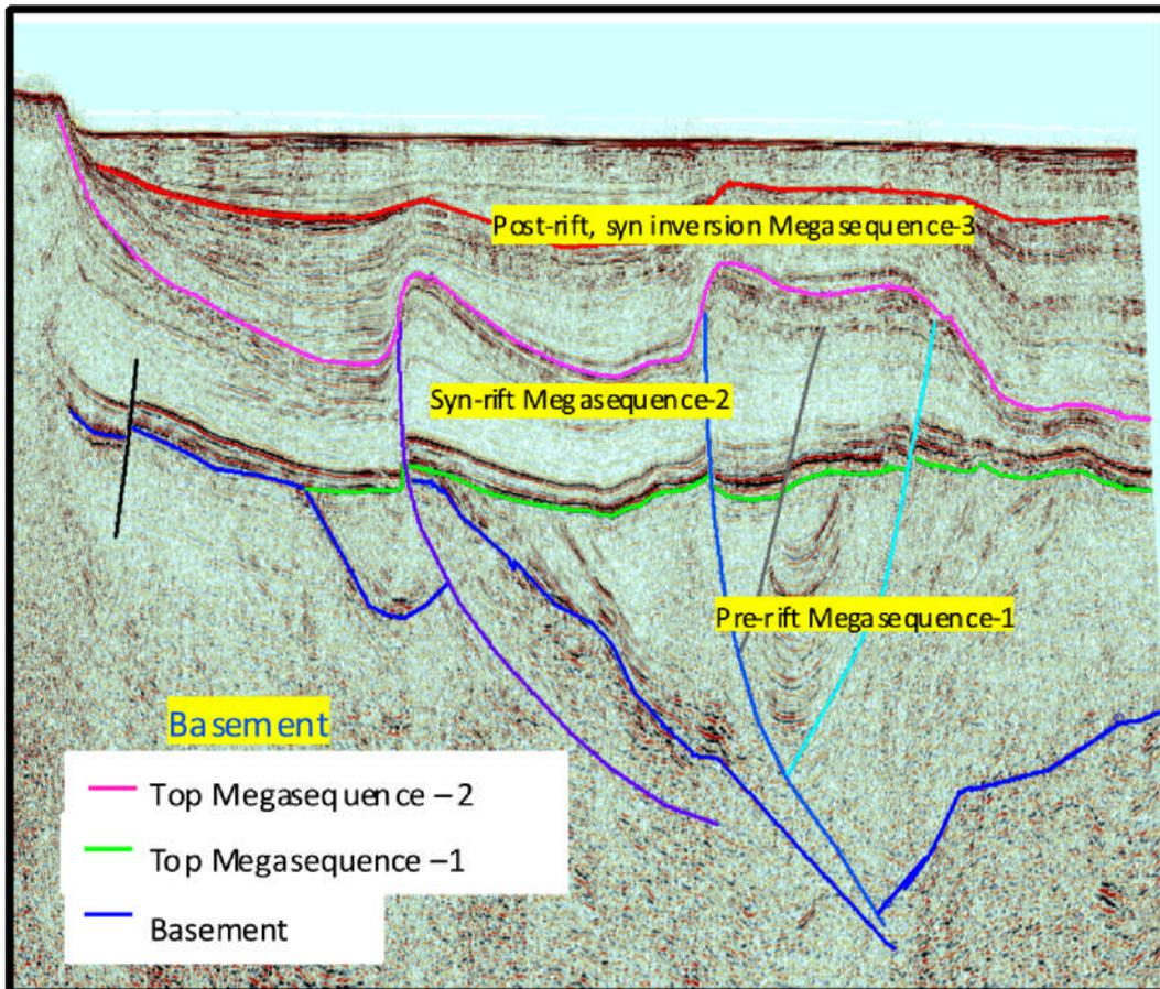
Figure 4 - Seismic section showing Pre-rift, syn-rift and post rift megasequences.
