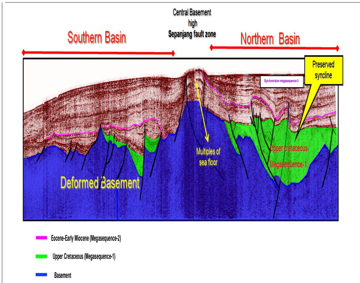
Figure 3 - N-S regional seismic line showing megasequences-1, 2 and 3.
